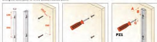
Drilling the wall to fix the surface-mounted profile.
