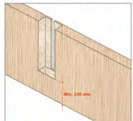
Dimensions for machining the wood panelling.
