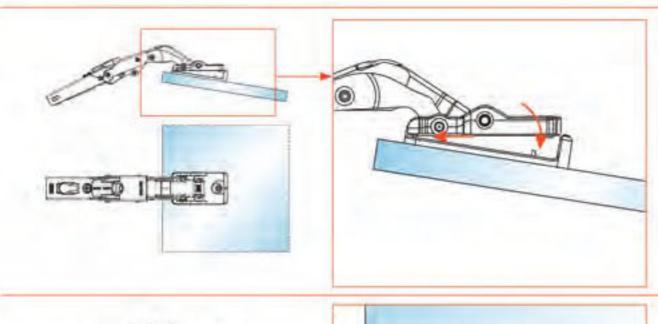
3) Rotate the fixing cam.
