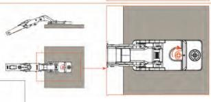
3) Rotate the fixing cam.
