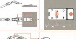
The hinge plate must be fixed to the door with the included screws.
