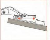
2) Locate the hinge onto the plate when it is fixed to the door.
